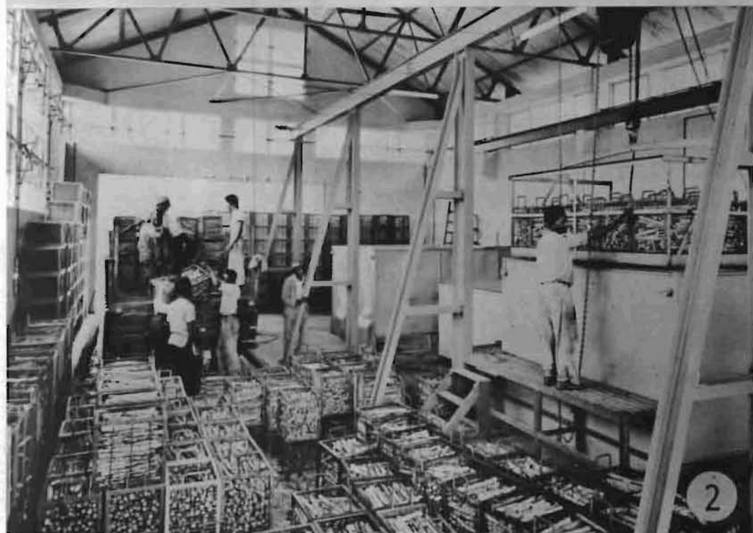
Fig. 21. Central hot water treatment plant of the M.S.P.A. at Belle Rive Experiment Station. (1) Exterior view of the building, (2) interior view showing baskets of cuttings and a cage being lowered in one of the two tanks; the fungicide tank is seen at the right centre.
