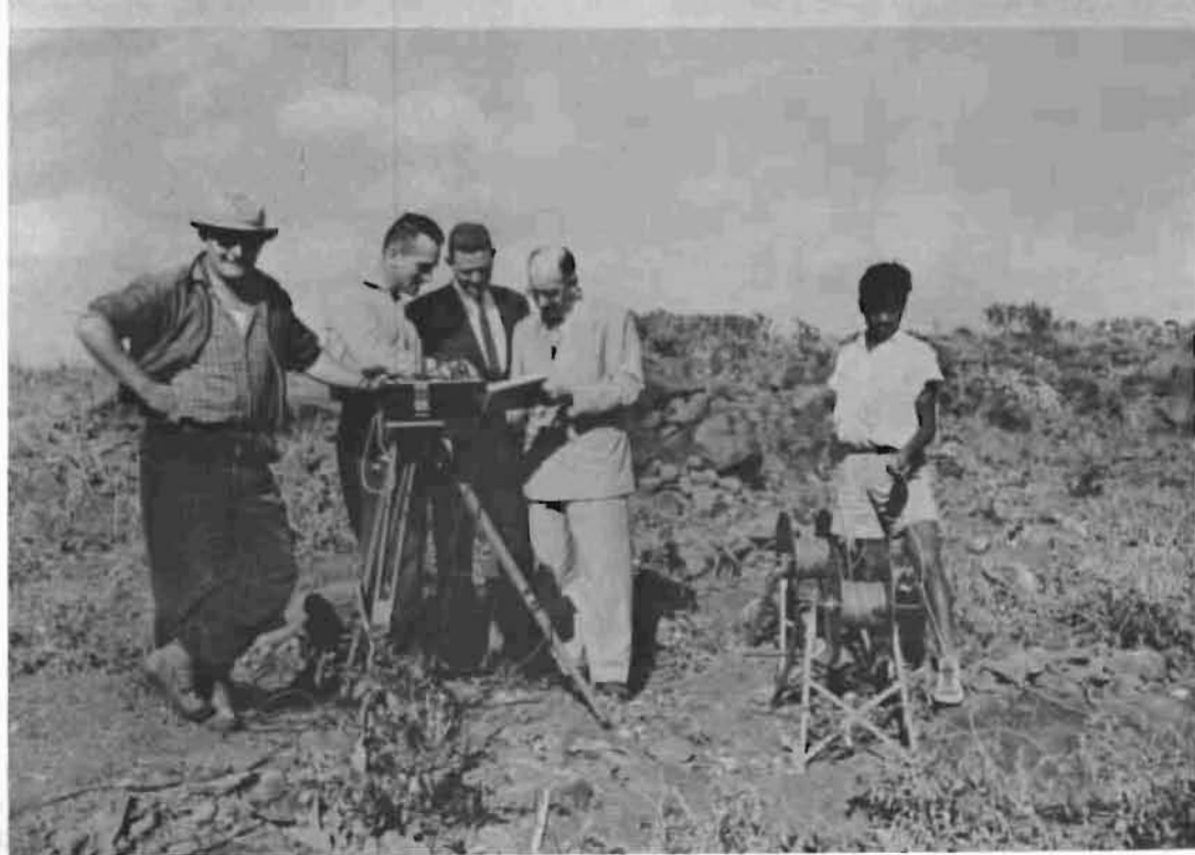
Fig. 37. Ground water survey in the Pamplémousses area by Schlumberger electrical resistance method.
