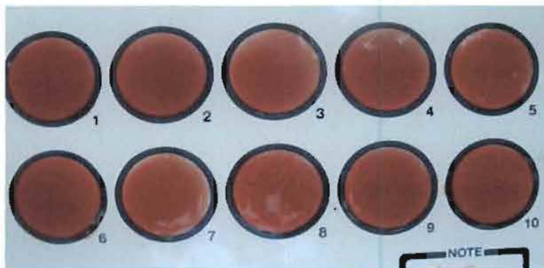
Figure 4 : Illustration du CATT effectué sur sang total (CATT/sg) (source IRD/CIRDES)
